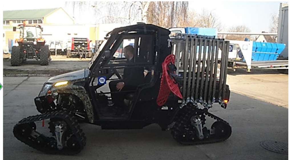
Tracked ATV – mini-tractor of biomass train
