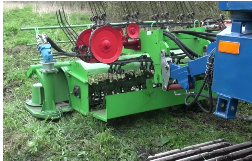
Real model of biomass conditioner with knives and flails
