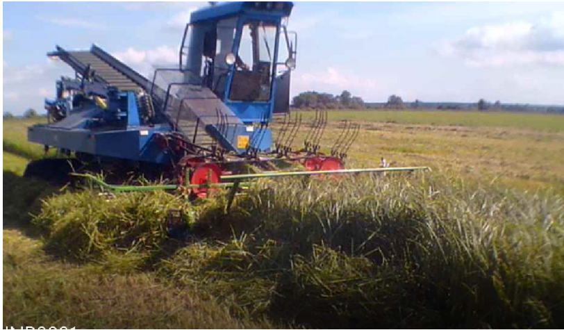
Mower unit - disk mower and finger-wheel rake and tedder
